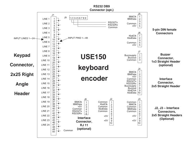
Figure 2 USE150 Connection Diagram
